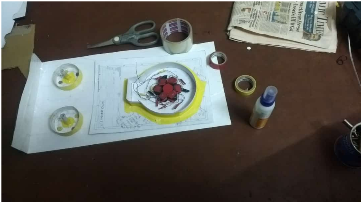
Fig 4,5 - Preparation of mould for casting, taping to reduce epoxy leakage
