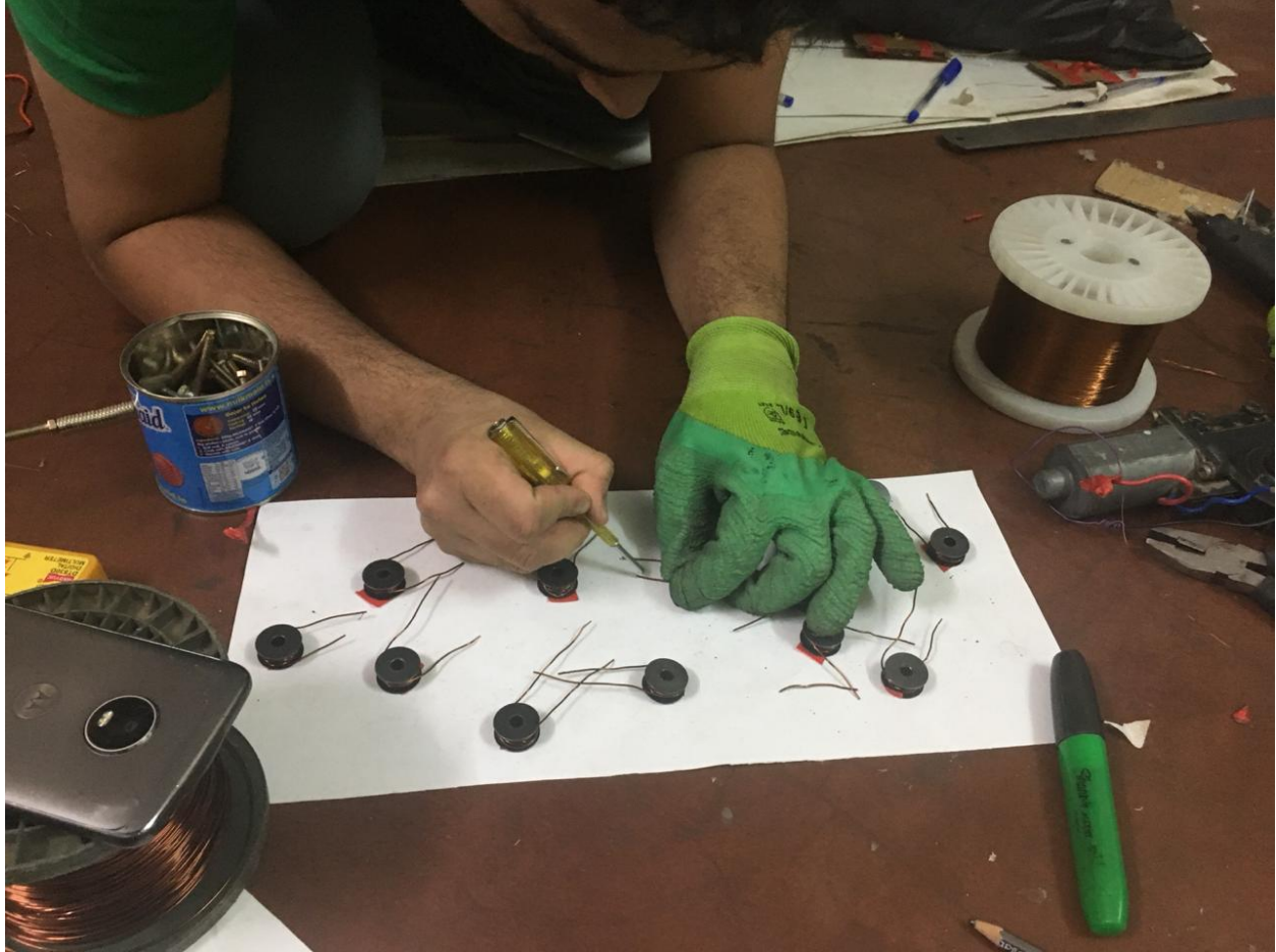
Fig 2 - Scraping of wire ends / removal of enamel
