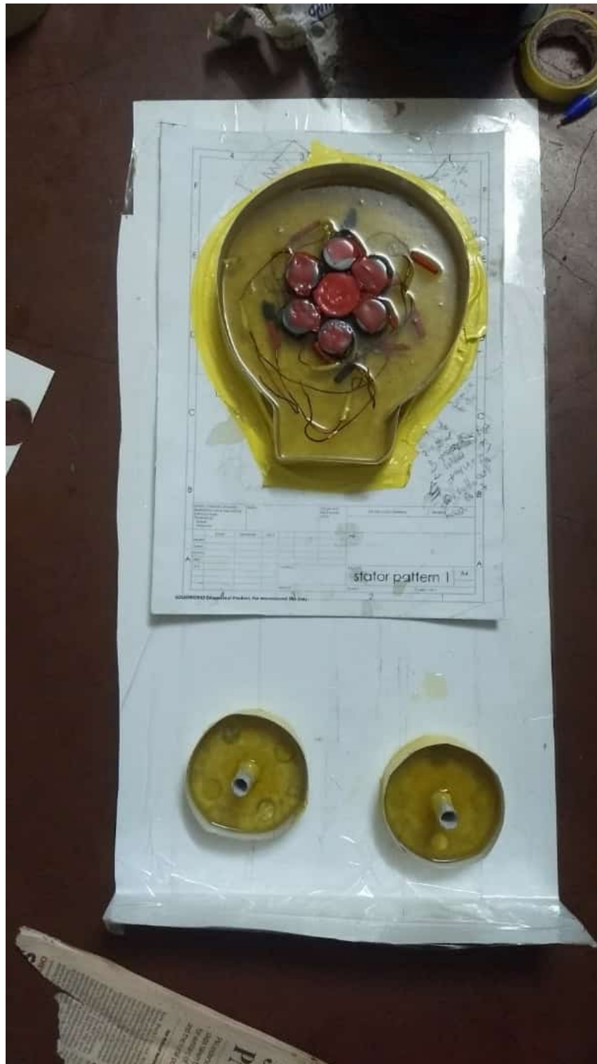
Fig 8 - Final cast with epoxy
