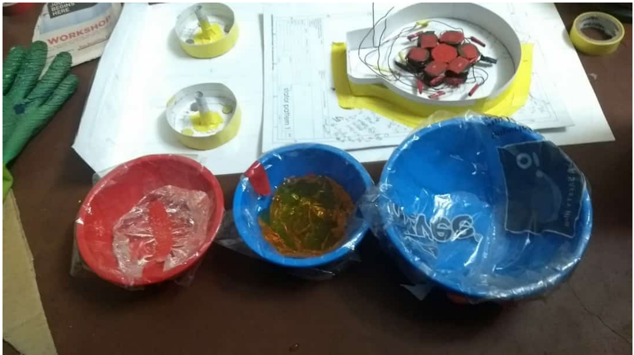
Fig 6,7 - Measurement and mixing of resin and hardener
